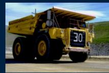
Simulate the movement of truck and shovel fleet to estimate the cycle times, mine throughput and utilization. Incorporate rimpull curve and haul route properties to validate mine plans and forecast operations down to a small variance from the real operations.
